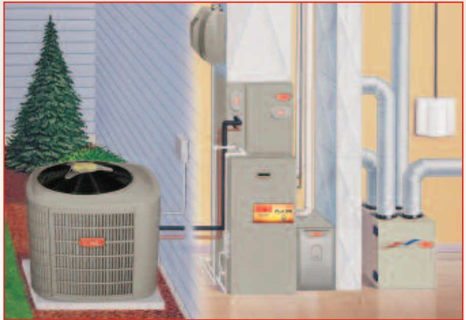
Air Conditioner and Gas Furnace System
